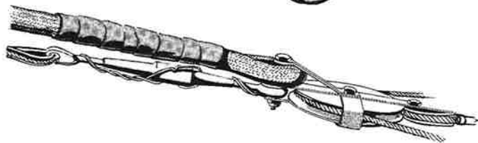
2. ADJUST TRAVEL OF SLIDE ON SLIDE TUBE BY TURNING TURNBUCKLE, LOCATED JUST AFT OF BAGGAGE COMPARTMENT, TO RIGHT OR LEFT.
